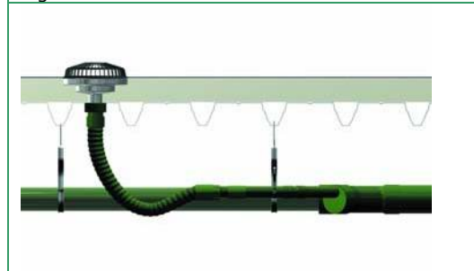
Fig 4: outlet connection may not sag underneath collector pipe
